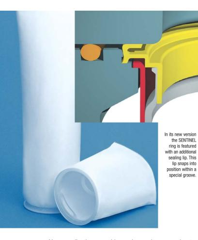
Now, applications requiring polypropylene or polyester felt filter bags can take advantage of the all-welded construction afforded by Eaton patented SENTINEL® Filter Bags. These bags, made from silicone-free materials, feature super-strong welded construction rather than sewn seams. This construction ensures that nothing bypasses the process media through holes in sewn fabric.
