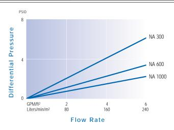
The graph indicates pressure drop versus flow rate of the various grades of Depth-Clear filter media in water. Adjustments may be required for other fluids. Please check with your Purolator representative for assistance in sizing.
