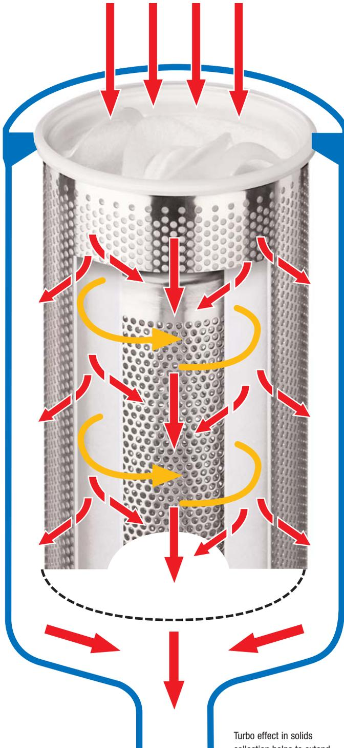
Turbo effect in solids collection helps to extend life of filter element
