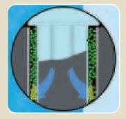
During backwash (triggered by time or pressure differential), a valve switches one station's flow from the inlet header to the drain header to facilitate reverse flow. Liquid is run in reverse through the system to remove contaminants from the media. Contaminants and cleaning fluid are expelled through the drain header at the base of the unit.
