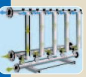
With an internal backwashing system, a small amount of clean process liquid flows backward through the tube being cleaned and out the drain header at the unit base.
